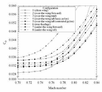
Fig. 22 Drag coefficients of all configurations.
